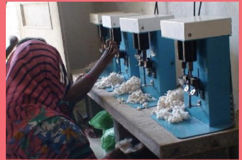
This machine was developed to automate the production of cotton wicks and increases the production efficiency of users by 400%, thus also augmenting a woman's capacity to earn. An entrepreneur has two options:
